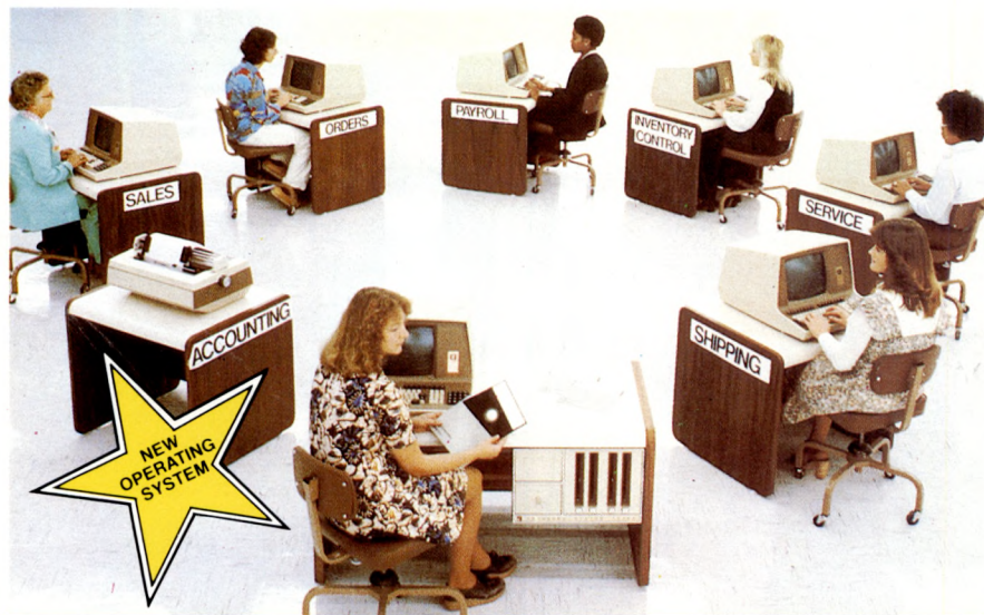
Multi-user System Three, with 320K memory, 4 discs, 7 terminals and fast line printer. Each terminal has its own operating system, and can run any software package independently.
